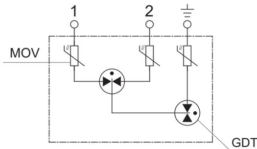
GDT: Gas-filled discharge tubes
